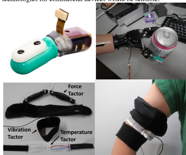
Figure 1: Top-Left: Multimodal BioTac tactile sensor, Top-Right: Prosthetic hand equipped with multimodal tactile sensors, Bottom-Left: Tactors, Bottom-Right: Tactors being worn.
